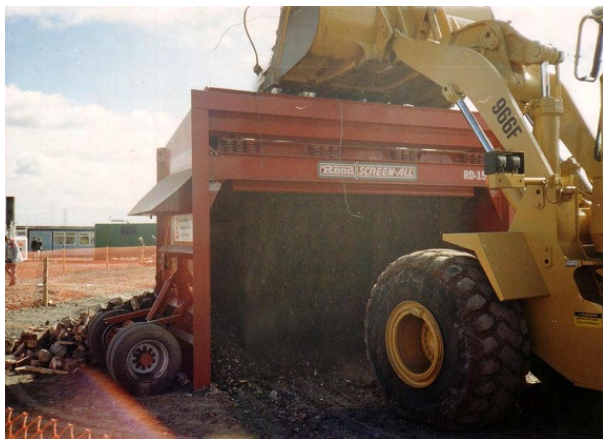
a) Loading stones onto vibrating screen
