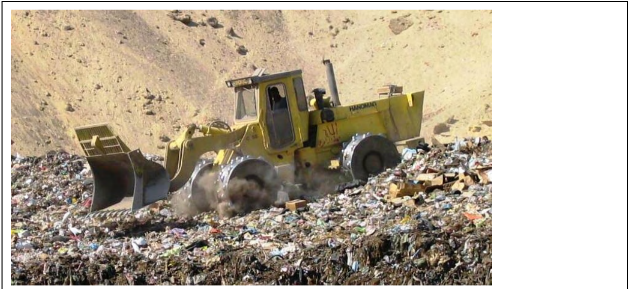
Photo B4.22 Landfill compactor fitted with a bucket instead of a bulldozer blade.
