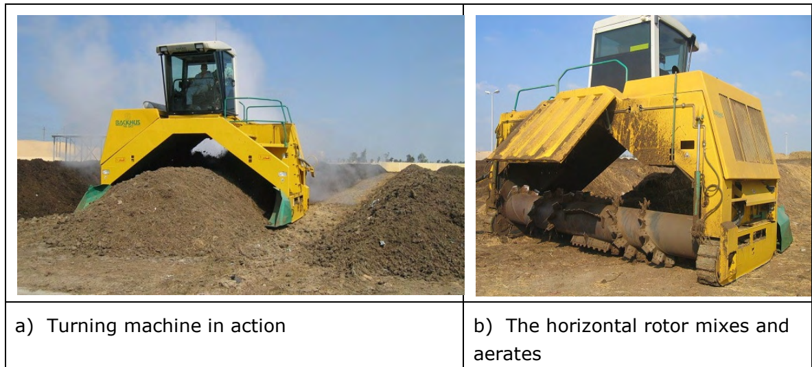
Photos C2.1 Windrow turning machine for mixing and aerating windrows in the early stages of composting
