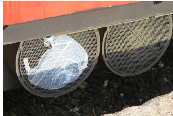
➤ d) Plastic bags can block screens, reducing the flow of air or water, or even damaging equipment. This screen is on a train.
