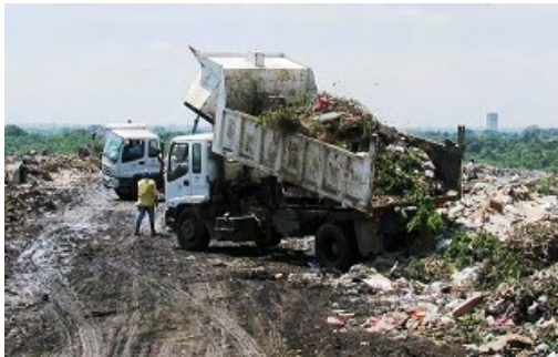
➤ a) If the access to the unloading area of the dump is like this, the vehicles bringing waste will experience many problems
