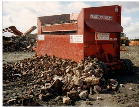
b) Coarse material falls outside the screen unit
