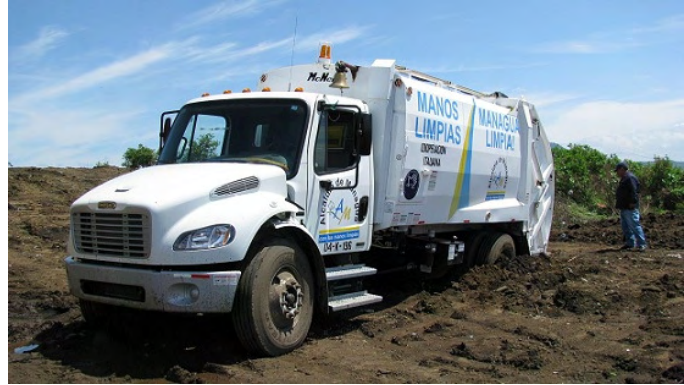
➤ b) When vehicles dig their rear wheels into soft ground they may damage their transmissions and there will be delays, as well as obstruction of other vehicles.
