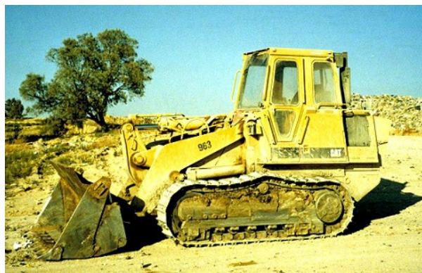
Photo B4.21 Small tracked loader with multipurpose bucket
