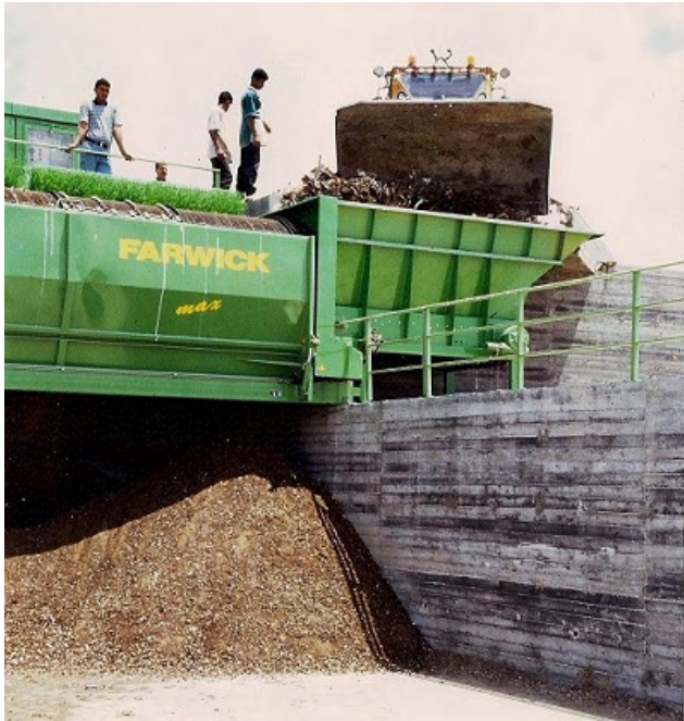
Figure C6.3 Fine material coming from the screening machine
