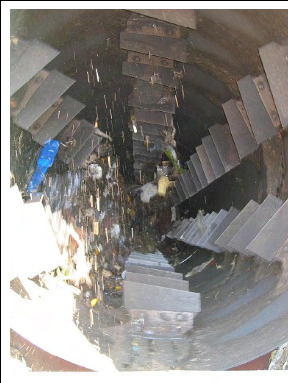
Photo C3.1 View inside a trommel
